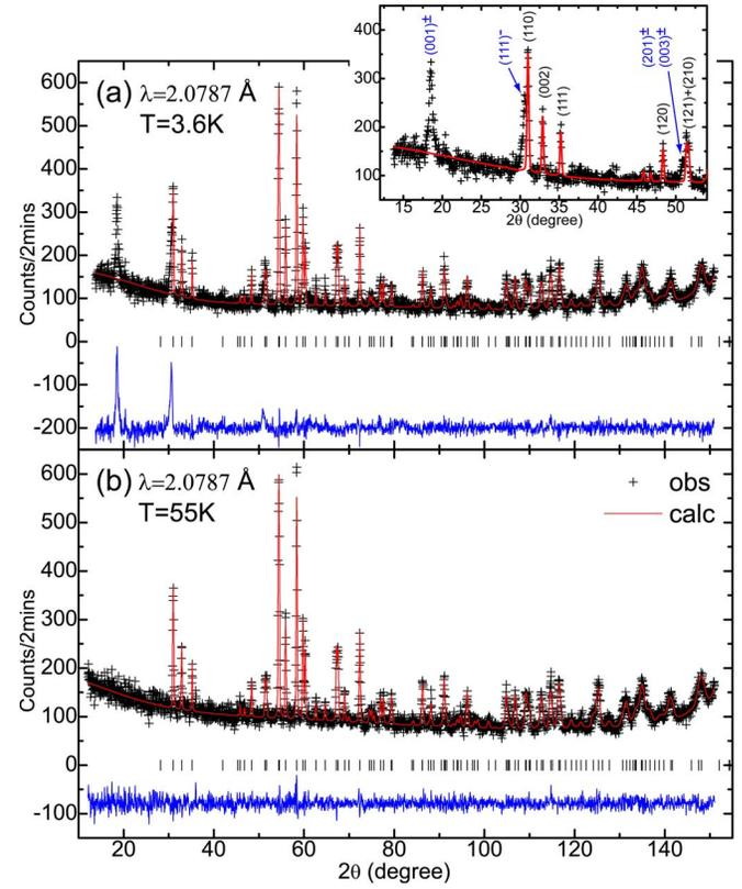
FIG. 2. (Color online) (a) High-resolution neutron powder diffraction pattern of the orthorhombic  $\text{ErMnO}_3$  specimen at (a) 3.6 K (below  $T_{N1}$ ) and (b) 55 K (above  $T_{N1}$ ). Inset zooms in on the lower-angle portion of the diffraction pattern, with the magnetic and structural reflections indexed.
