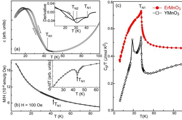
FIG. 1. (Color online) Temperature dependence of (a) the dielectric constant  $\varepsilon(T)$ , (b) the magnetization  $M(T)$ , and (c) the specific heat  $C_p(T)$  of the orthorhombic  $\text{ErMnO}_3$ . Inset shows the  $T$  derivative of  $\varepsilon(T)$  in the lower temperature range.  $C_p(T)$  data for the orthorhombic  $\text{YMnO}_3$  (similar to the work reported by Kim *et al.* 19) are also plotted for comparison.
