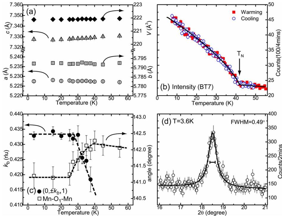
FIG. 3. (Color online) Temperature dependence of (a) the lattice parameters  $a$ ,  $b$ ,  $c$ , and cell volume  $V$ , (b) the peak intensity of  $q = (0, \pm k_b, 1)$ , and (c) the  $k_b$  component of the propagation wave vector and the Mn-O<sub>1</sub>-Mn bonding angle. (d) The scattering profile near  $q = (0, \pm k_b, 1)$  at  $T = 3.6$  K.
