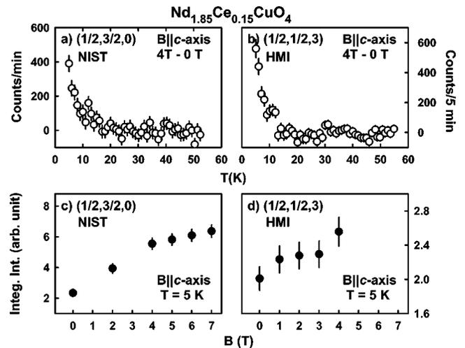
FIG. 9. Comparison of the field-induced effect for superconducting  $\text{Nd}_{1.85}\text{Ce}_{0.15}\text{CuO}_4$  at  $(1/2,3/2,0)$  and  $(1/2,1/2,3)$ . While the data at  $(1/2,3/2,0)$  are from Ref. 29, the results at  $(1/2,1/2,3)$  are new, to our knowledge. The temperature dependence of the difference between 4 and 0 T at (a)  $(1/2,3/2,0)$  and (b)  $(1/2,1/2,3)$ . The field dependence of the integrated intensity at (c)  $(1/2,3/2,0)$  and (d)  $(1/2,1/2,3)$ .
