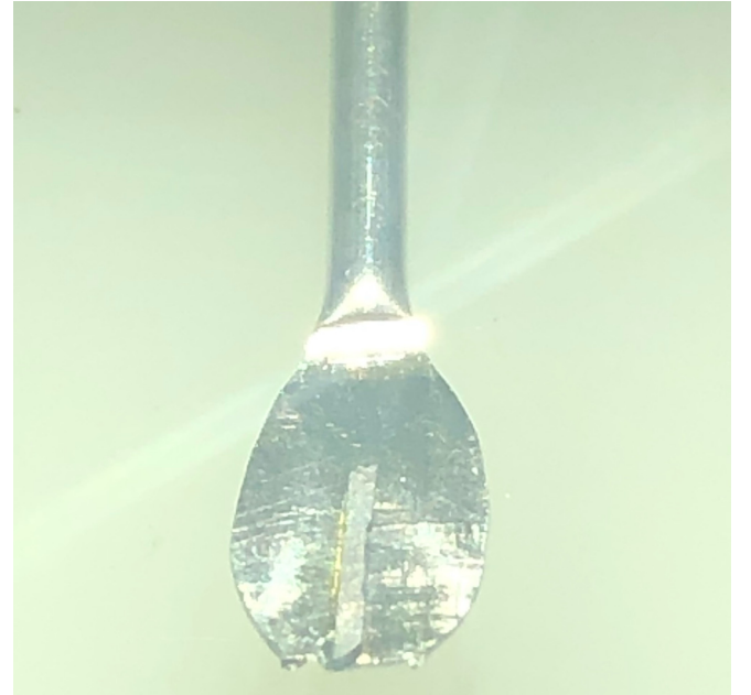
FIG. 12. Photograph of the \text{Eu}(\text{Ga}_{1-x}\text{Al}_x)_4 with x = 0.9 sample measured during CORELLI measurements. Due to the large absorption of Eu, a single-crystalline piece of \text{Eu}(\text{Ga}_{1-x}\text{Al}_x)_4 with x = 0.9 sample was cut into a thin rod, as shown. Therefore, as the sample was rotated 360^\circ to collect a reciprocal-space map, a uniform cross section was irradiated with neutrons.
