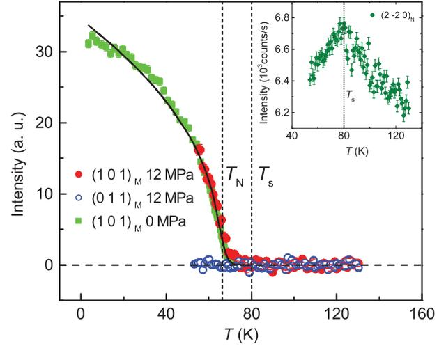
FIG. 1. Temperature dependence of the intensity of the AF Bragg peaks at  $(1\ 0\ 1)$  and  $(0\ 1\ 1)$  under 0 and 12 MPa. The solid line is fitted as described in the text.  $T_N$  is determined from the fitting. The inset shows the temperature dependence of the intensity of the nuclear Bragg peak at  $(2\ -2\ 0)$ , which shows a kink at  $T_s$ .
