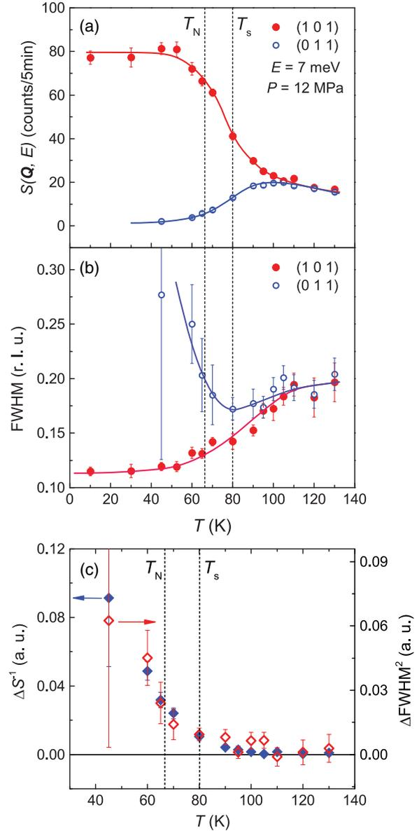
FIG. 3. Temperature dependence of (a)  $S(\mathbf{Q}, E)$  and (b)  $\text{FWHM}$  at  $(1\ 0\ 1)$  and  $(0\ 1\ 1)$  at 7 meV and 12 MPa. (c) Temperature dependence of  $\Delta S^{-1}$  (blue solid diamonds) and  $\Delta \text{FWHM}^2$  (red open diamonds) as defined in the main text. The solid lines are a guide for the eye. The vertical dashed lines indicate  $T_s$  and  $T_N$ . The error bars are given by the Gaussian fits.
