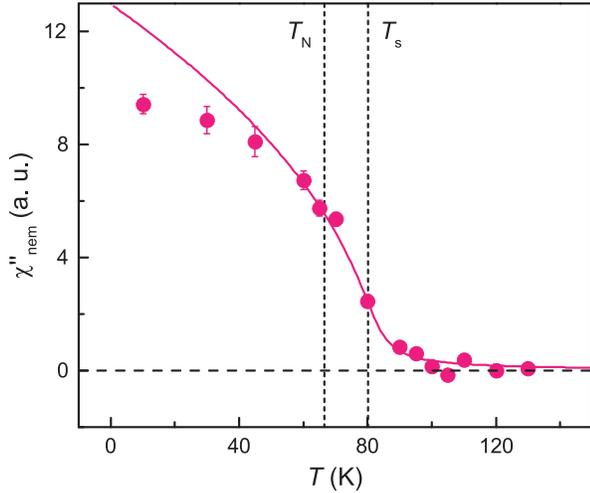
FIG. 4. Temperature dependence of  $\chi''_{\text{nem}}$ . The solid line is calculated according to the Landau free energy as described in the main text with  $a_0 = 3.73$ ,  $b = 0.036$ , and  $h = 266$ . The vertical dashed lines indicate  $T_s$  and  $T_N$ .
