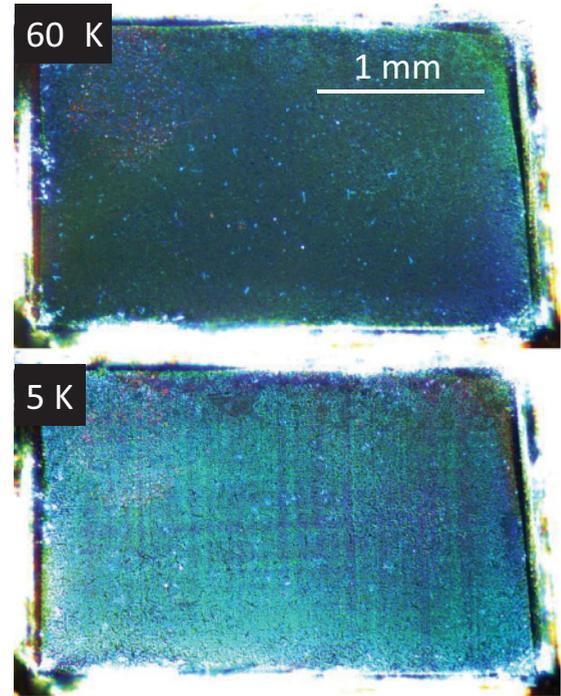
FIG. 8. (Color online) Polarized-light images of the fresh cleaved surface of a  $\text{Na}_{1-\delta}\text{FeAs}$  sample, taken above structural transition at 60 K (top panel) and at 5 K, the base temperature of our experiment (bottom panel). The image shows a pattern of structural domains with domain walls running along the [100] tetragonal direction.
