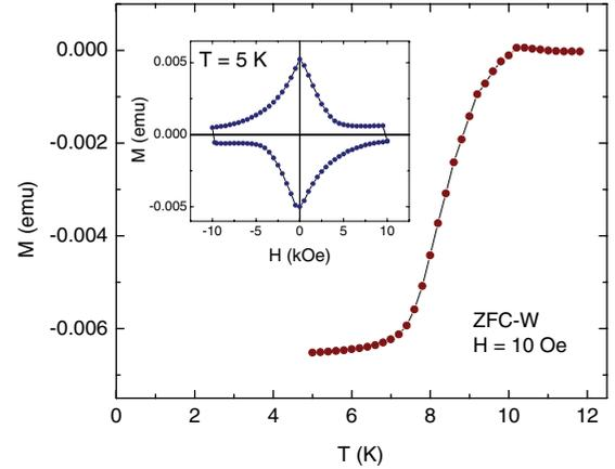
FIG. 2. (Color online) Direct current magnetization of fresh cleaved sample measured upon warming after cooling in zero magnetic field and applying a 10 Oe field (ZFC-W). Inset: magnetic hysteresis loop measured at 5 K in the same sample.
