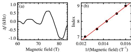
FIG. 3 (color online). (a) PDC resonant frequency for a  $\text{YBa}_2\text{Cu}_3\text{O}_{6.69}$  crystal after background subtraction to leave the oscillatory component  $\Delta f$ ; the trace is a smoothed average of three magnet sweeps ( $T = 1.5$  K). (b) Oscillation index versus reciprocal magnetic field for the MQOs in (a) (points); dips in  $\Delta f$  are indexed by integers and peaks by half integers. The straight line is a fit with a gradient of  $550 \pm 20$  T.
